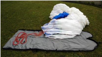
Sit on the opposite side of the bag and pull the cells onto the bag, one by one, from the nearest stable, across the middle and to the furthest stable.
